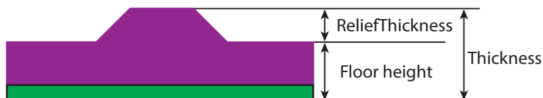
Figure 8-36: Relief and floor thickness for a flexo plate or flexo sleeve
