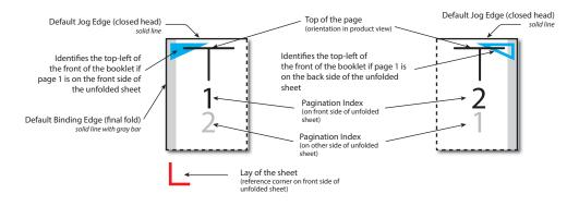
Folding sequences are described using the same notation found in ▶ Section A.3.8 Fold Catalog.
