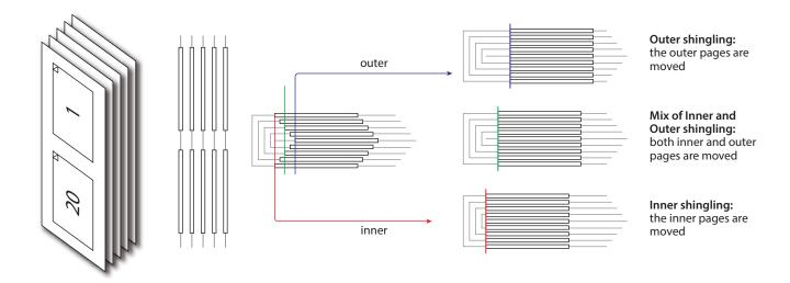
Figure 6-25: Shingling for stripping – details
