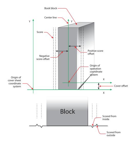
Figure 6-12: Parameters and coordinate system for glue application
