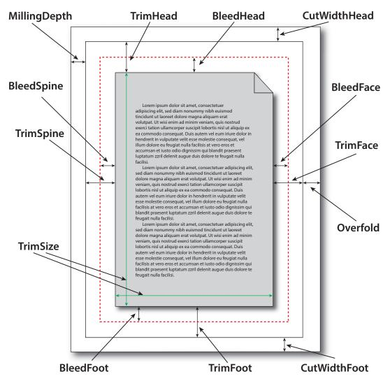
**Note:** Overfold in this figure refers to the value of the parent **BinderySignature**/@Overfold and is only present if the page requires an overfold based on the value of the parent **BinderySignature**/@OverfoldSide.
