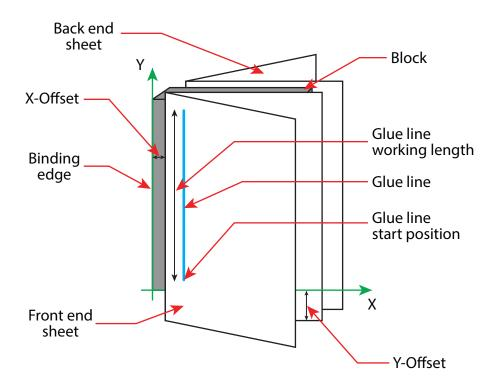
The process coordinate system is defined as follows: The Y-axis is aligned with the binding edge of the book block. It increases from the registered edge to the edge opposite to the registered edge. The X-axis is aligned with the registered edge. It increases from the binding side to the face side opposite the binding side.
