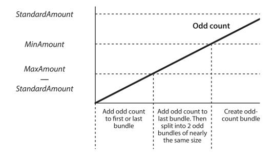
Figure 5-12: Odd count handling for a layer
