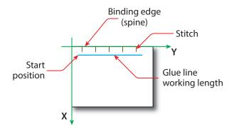
Figure 6-43: Parameters and coordinate system used for side sewing
