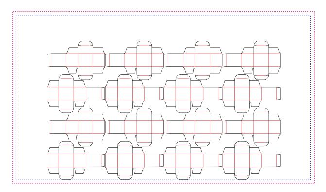
In the following figure, 1-ups on even columns are rotated 180 degrees. Even columns are shifted vertically and horizontally to obtain optimal nesting.
