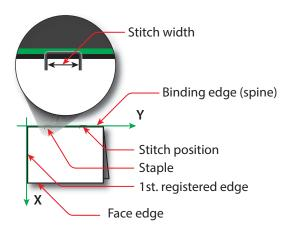
Figure 6-38: Parameters and coordinate system used for stitching
