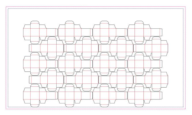
In the following figure, 1-ups on even rows are rotated 180 degrees. Even rows are shifted vertically to obtain optimal nesting. The even rows are not shifted horizontally (left and right edges are aligned between rows).
