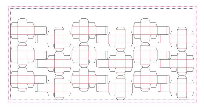
In the following figure, 1-ups on even columns are rotated 180 degrees. Even columns are shifted horizontally to obtain optimal nesting. No vertical shifting of even columns is done (top and bottom edges are aligned between columns).
