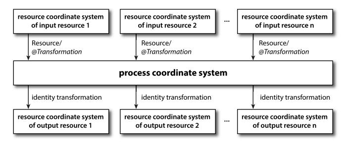
It is important that no implicit transformations (such as rotations) are assumed if the dimensions of the input resources of a process do not match each other. Instead every transformation (e.g., a rotation) SHALL be specified explicitly by using the **Resource**/@Orientation or **Resource**/@Transformation.
