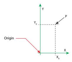
Each page contained in a PDL file has its own coordinate system. In the same way a piece of film or a sheet of paper has a coordinate system. Within **XJDF** each of these coordinate systems is called a *resource coordinate system*.
