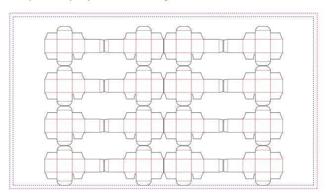
In the following figure, @LayoutStyle = "Reverse2ndRow", @GutterX = "36", @GutterX2 = "70", @GutterY = "20", @GutterY2 = "40".
