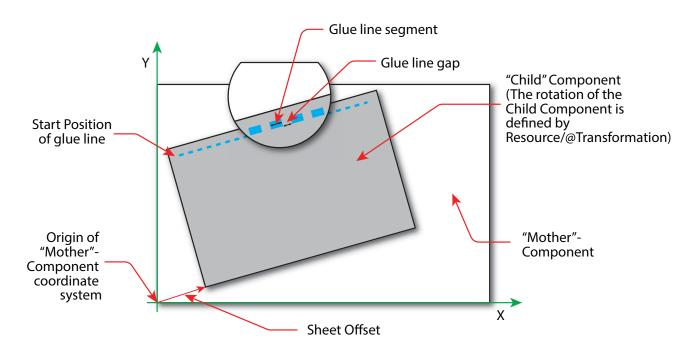
The process coordinate system is defined as follows: The Y-axis is aligned with the binding edge and increases from the registered edge to the edge opposite the registered edge. The X-axis, meanwhile, is aligned with the registered edge. It increases from the binding edge to the edge opposite the binding edge, which is the product front edge.
