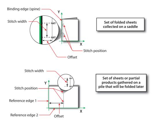
Figure 6-39: Stitching coordinate system for aStitchOrigin values
